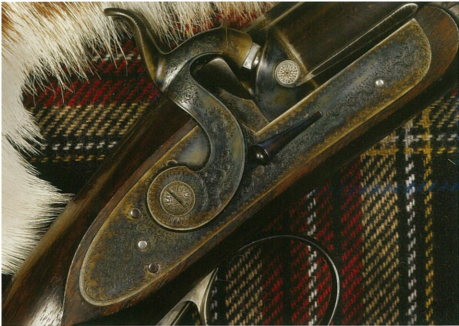
The lock of no.3795 showing the flat hammer and fine scroll engraving.
