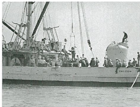
The rescue chamber aboard the Falcon. Photo courtesy Boston Public Library Leslie Jones Collection.
