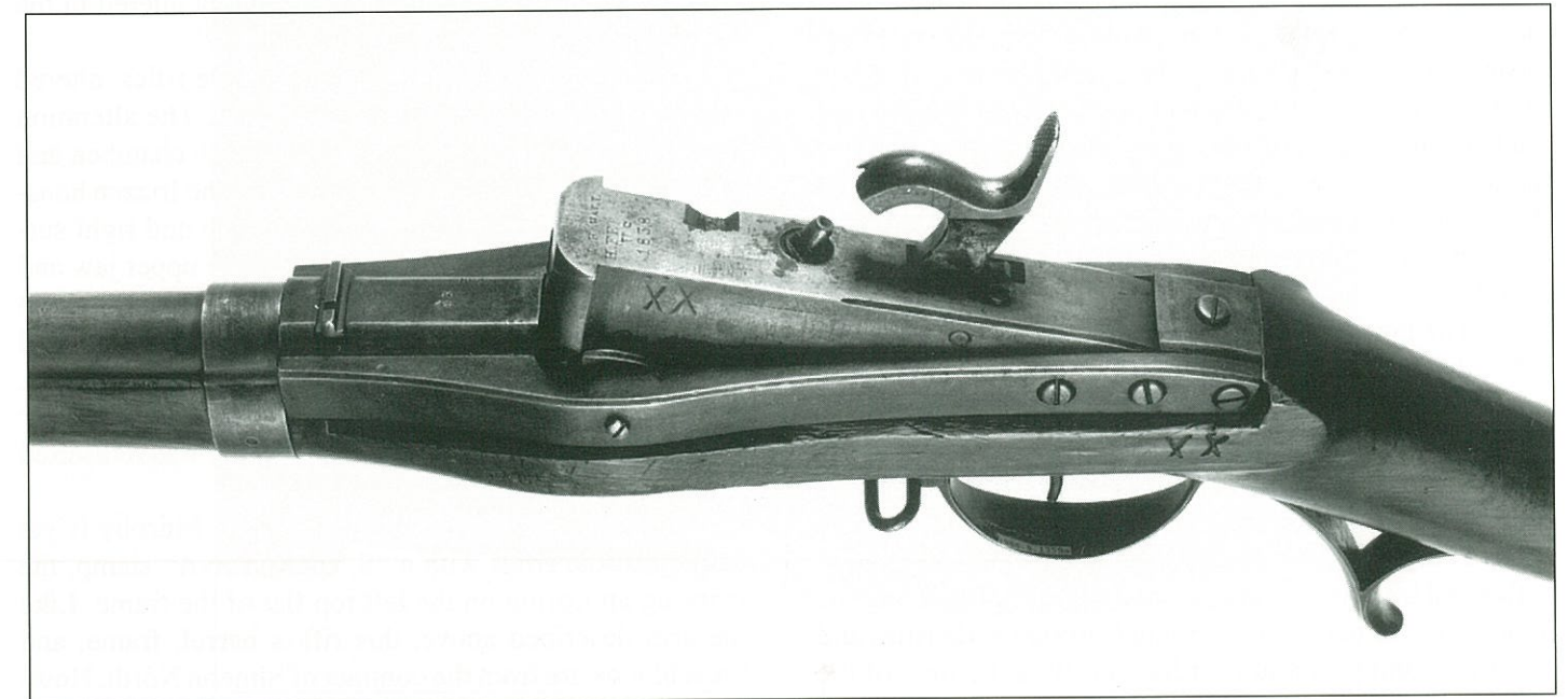
Plate 3. Close-up view of breech area of the rifle illustrated in Plate 1, showing Roman numeral marking "XX" on side of breechblock and original Hall's markings on top. (Courtesy Cody Firearms Museum, Buffalo Bill Historical Center)
