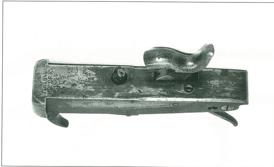
Plate 15. Close-up view of an "1824"-dated Hall's patent rifle breechblock, showing method of percussion alteration and newly-made hammer. (Courtesy Springfield Armory Museum, Milwaukee Public Museum photograph)
