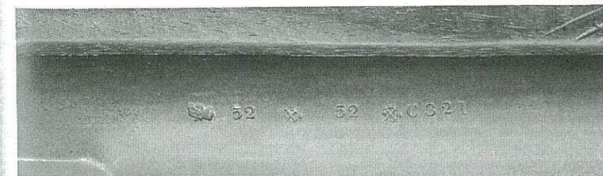
The left side of the barrel this rifle, No. "C 321", showing the number, Birmingham proofs and .52 bore.
