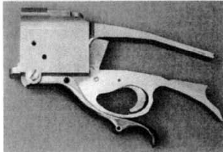
Danie's Farquharson action in different stages of production. They used Böhler M200 steel.
