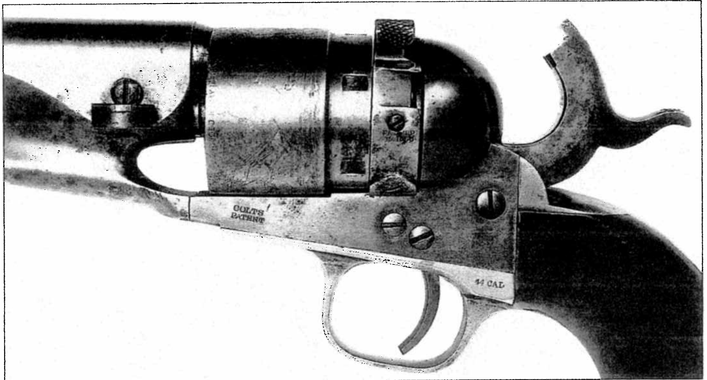
Fig. 4-68 Close-up of 1860 Army Thuer conversion action showing markings. Serial number 178577.
