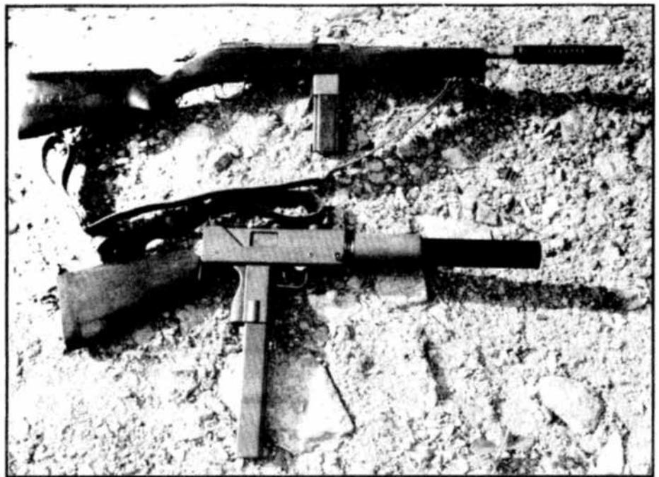
The Reising submachine gun with Maxim silencer is lighter, quieter and handier than the Ingram M10 .45 cal submachine gun with SIONICS suppressor, and it has four times the effective range.
