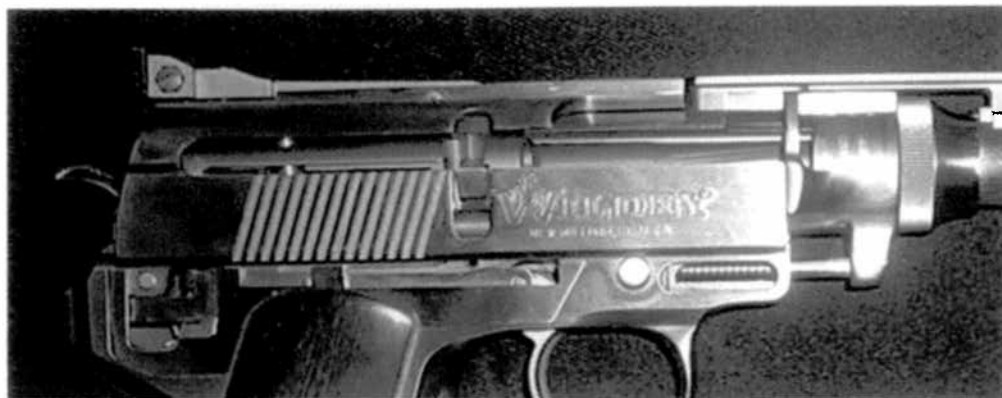
Factory cut-out Wildey pistol, showing the locking system and trigger linkage
