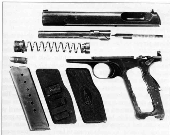
Figure 14: .45 ACP pistol stripped. Note the flat rectangular section main spring and the two-part locking lug around the breech — the helical section mates with the cam in the frame to control barrel rotation while the square section locks by engagement with the slide cutout.
