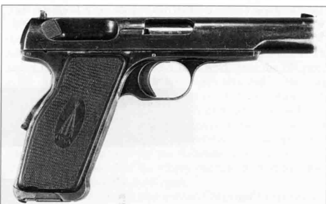
Figure 7: .45 ACP BSA pistol, right side. Note Birmingham proof marks on barrel and rear of frame.
