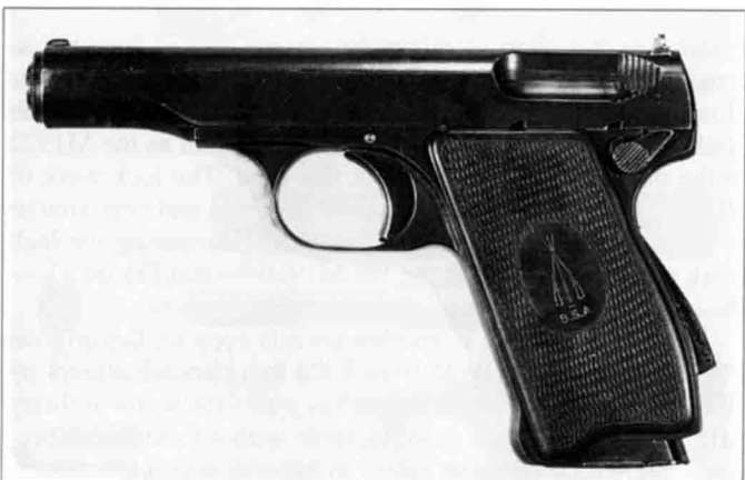
Figure 4: .34 Belted BSA pistol, left side. Note 'COCKED' on grip safety and gripping cuts in slide.
