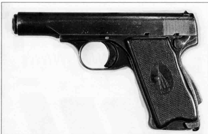
Figure 2: .32 ACP BSA pistol, left side. Note the 'COCKED' inscription on the grip safety and conventional finger gripping serrations to slide.
