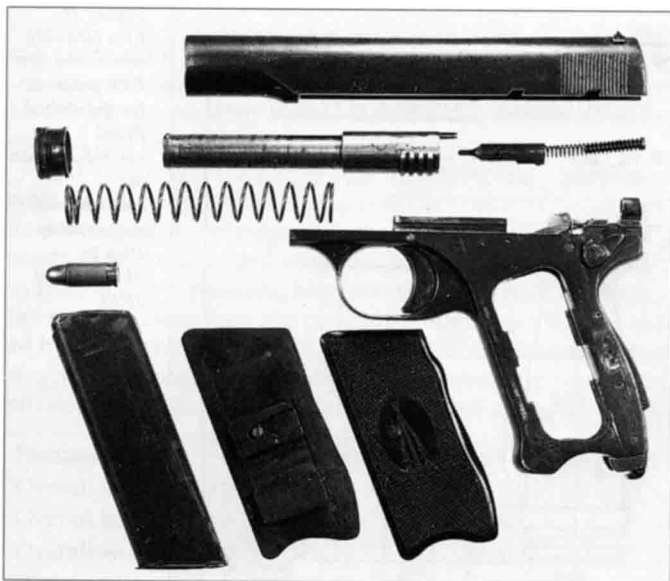
Figure 12: .32 BSA pistol stripped. Note the grip plate retaining dovetail lugs and spring.
