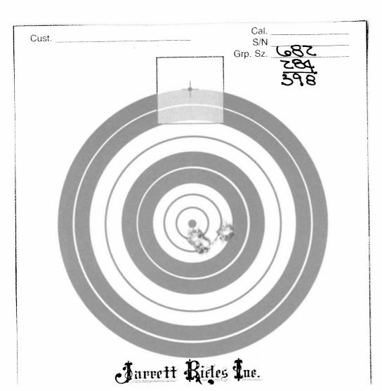
BULLET WT 150 gr., MUZZ.VELO. 3141 fps, BALL.COEF .429 , ZEROS AT 31 & 237 ydTRAJ HT.=+ 2.29 in.AT MIDRANGE 137 yd, - 2.29 in.AT POINT BLANK RANGE 277 yd RANGE (yd
