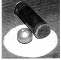
We stuffed a ball down the bore with a patch, and placed extra wads on the charge to eliminate air space. We got very fine accuracy from the old rifle this way. The rifle needs the right bullets to shoot to its potential.
