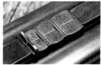
The leaves are labeled 200, 250, and 300. The height of the 300-yard leaf is in keeping with the rainbow trajectory of the rounds. The platinum center lines were very helpful in getting a sight picture with the shallow V.
